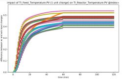
Explainable AI features assist APC engineers to validate models and sub-models based on engineering and process knowledge. The simulated behavior shows key characteristics of model leaning: Steady state gain range, time to steady state variation, and process delay.
